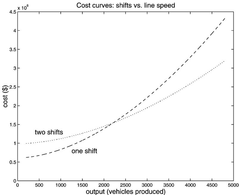
Fig. 1. Cost conditional on running one shift,  $C(q,1)$ , and running two shifts,  $C(q,2)$  holding hours per shift fixed.
