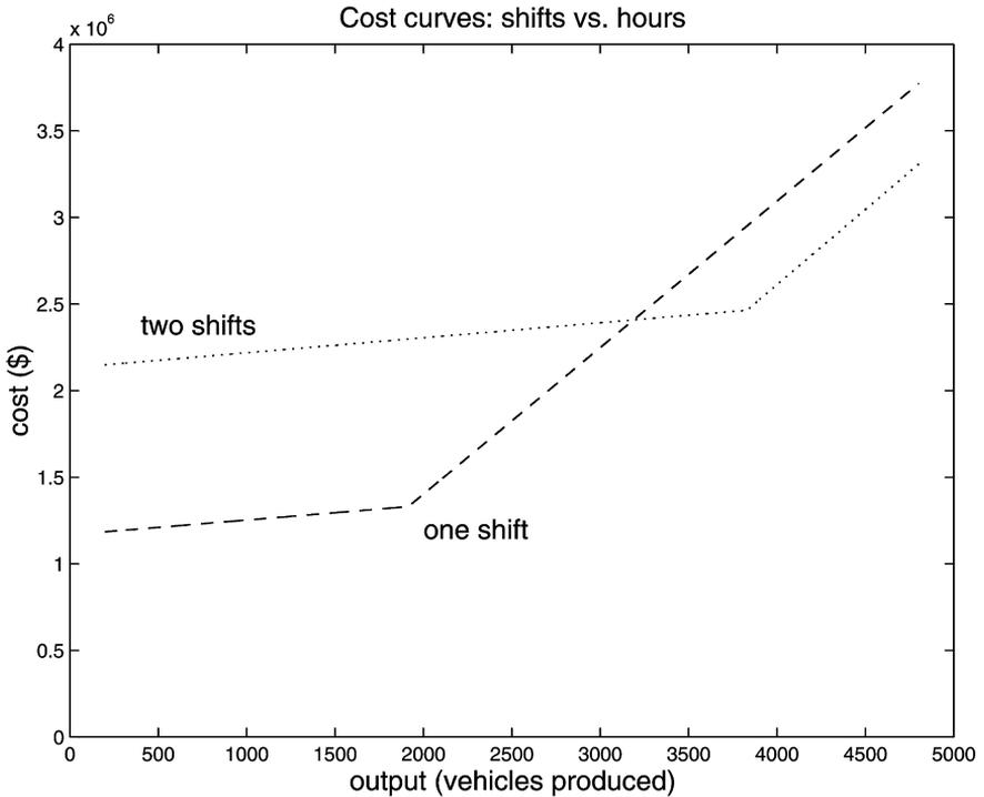
Fig. 3. Cost conditional on running one shift,  $C(q,1)$ , and running two shifts,  $C(q,2)$ , holding employment fixed.
