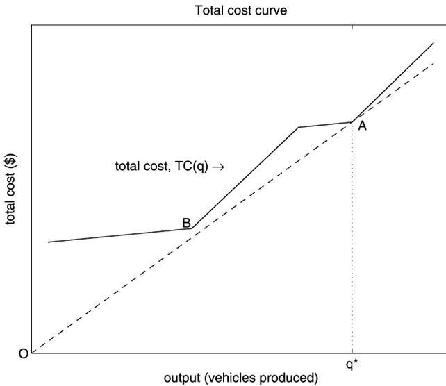
Fig. 4. Total cost curve allowing either one or two shifts to run,  $TC(q)$ , holding employment fixed.  $q^*$  denotes the minimum efficient scale (MES).
