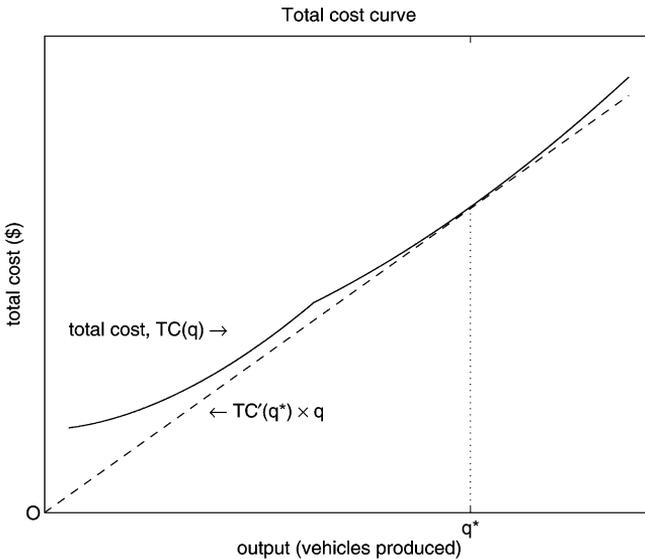
Fig. 2. Total cost allowing either one or two shifts to run,  $TC(q)$ , holding hours per shift fixed.  $q^*$  denotes the minimum efficient scale (MES).
