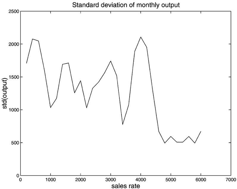
Fig. 12. Standard deviation of monthly output as a function of the weekly sales rate.
